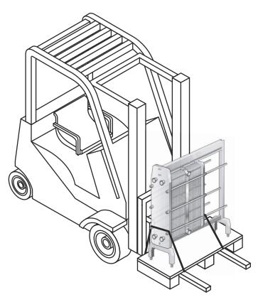
Before loosening the equipment from the pallet, secure the equipment from falling using hoist slings.
