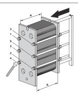
7 Tighten the four bolts (1), (2), (3), (4) or the six bolts (1), (2), (3), (4), (5), (6) evenly until **A** measure has been reached.
