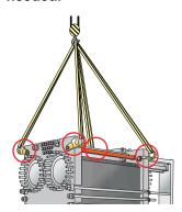
Figure 7: Lifting device for T50. Securing equipment is needed.
