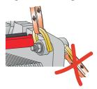
Figure 8: Lifting device for TS50. Use the four inner eyes when lifting the plate heat exchanger. Do NOT use the transport securing points! Securing equipment is needed.
