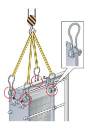
Figure 5: Lifting device for T35 and TS35. Securing equipment is needed.
