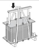
Place a hoist sling around one bolt on each side.
