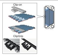
Repeat the procedure on all the plates that needs to be regasketed. Close the plate heat exchanger according to *Closing* on page 60.
