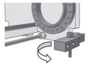
Loosen and remove the locking bolts. Identify them according to *Bolt configuration* on page 52.
