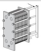
7) Mark the plate assembly on the outside with a diagonal line.
