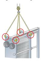
Figure 6: Lifting device for T45, TL35 and WideGap 350. Securing equipment not needed.
