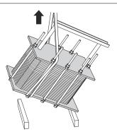
6 Lower the plate heat exchanger into a horizontal position and place it on the floor.
