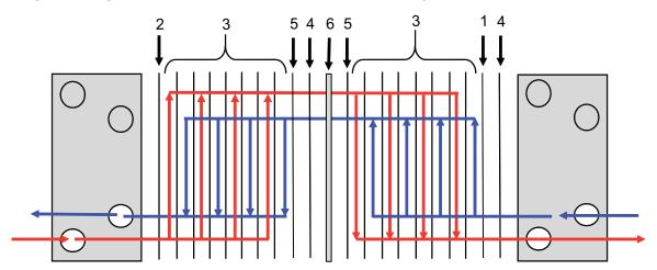
Figure 3: Example of a multi-pass set up.
