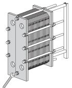
Use the tightening bolts, equipped with bearing boxes, to open the plate heat exchanger. During the opening procedure, keep the frame plate and pressure plate parallel. Skewing of the pressure plate during opening must not exceed 10 mm (2 turns per bolt) across the width and 25 mm (5 turns per
