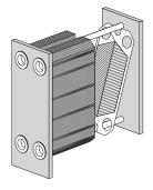
5 If the plate pack has been marked on the outside, check this according to Procedure Opening - Procedure. If the plates are correctly assembled (A/B/A/B etc.), the edges form a "honeycomb" pattern, see picture.
