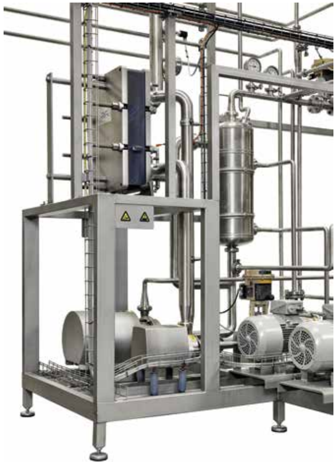
The de-alcoholization module's condensate cooling section
